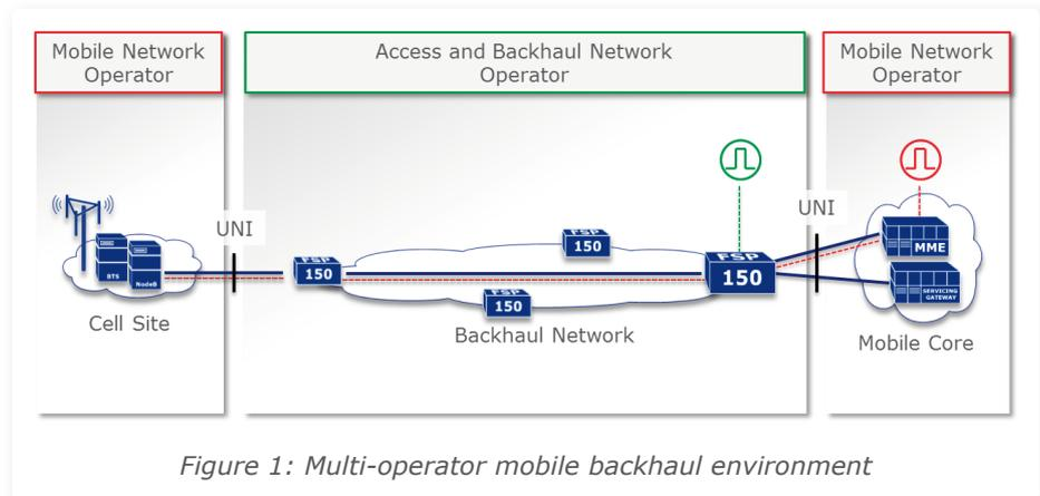
Figure 1: Multi-operator mobile backhaul environment
